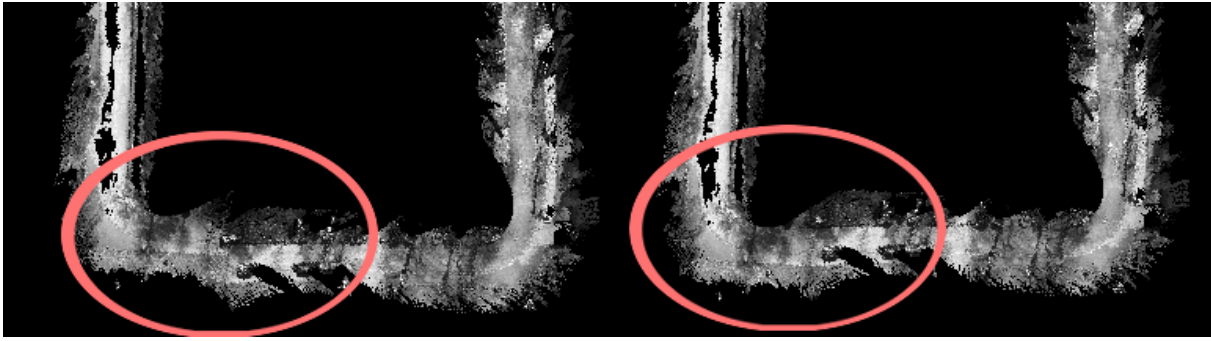
Fig. 5: The bottom part of the dense map before (left) and immediately after (right) closing the loop. A slight miss alignment can be observed on the left bottom of the loop. After loop closure this miss alignment is successfully resolved. The position of past poses is shown in Figure 4.
